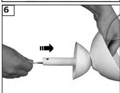
Place canopy and then yoke cover on downrod. Thread leadwires and safety cable through downrod. As shown.
